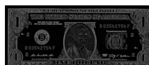
Figure 8: Sobel Filter used from Skimage Library gave similar results to that of the Canny Filter
