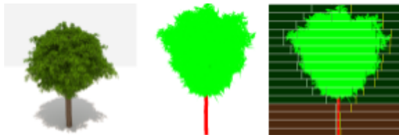
Figure 2. Generated tree, semantic mask (imposter), visualization of the division into stripes.
