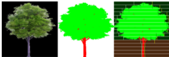
Figure 1. The original image, semantic mask, visualization of the division into stripes. Stripes of brown color correspond to the trunk, green color to the crown. Vertical lines inside each stripe - values a_i , b_i , c_i , d_i respectively.
