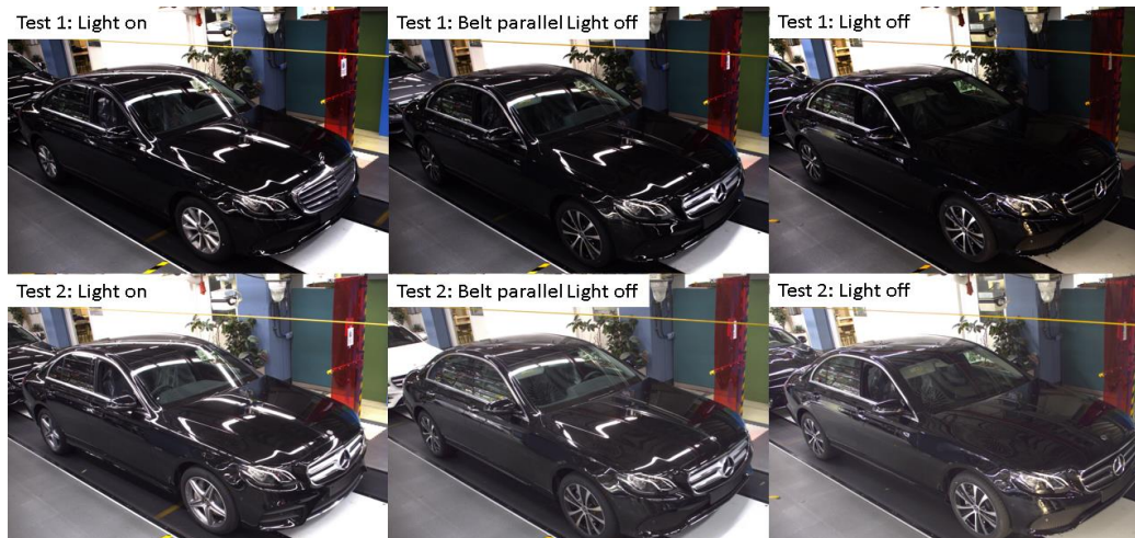
Figure 2: Tests with light turned on, belt parallel lights turned off and light in the station turned off. Top row: Unmodified images. Bottom row: Images with automatic color and contrast correction.
