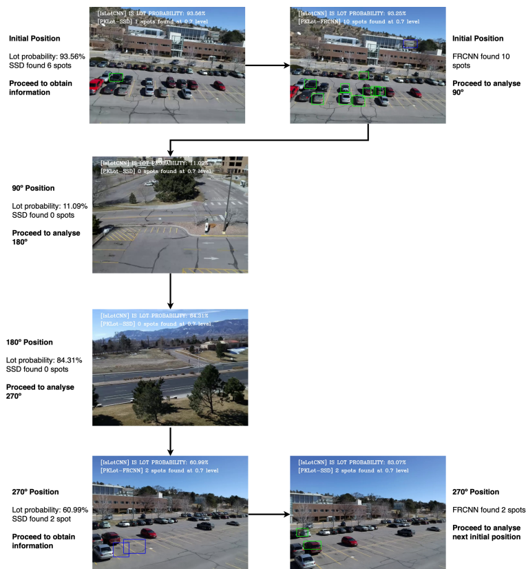
Figure 5: Flight test with FRCNN Resnet50 and SSD Inception
