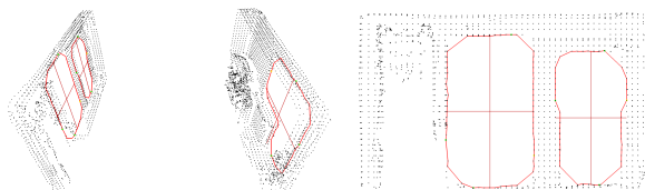
Figure 6: Localization of relevant objects for a comparison of differences using \alpha -shapes in the planar point cloud of the extracted wall sides by the amplitudes of the mass histogram.
