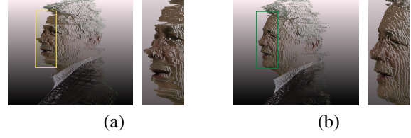
Figure 5: Resulted point cloud of a real actor "Jacques". (a) point cloud obtained with integer disparity values without VH guidance and zoom in its yellow area. (b) point cloud obtained with integer disparity values with VH guided stereovision and zoom in its green area.
