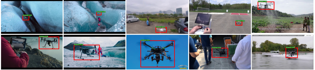
Figure 6: Some of our test images. UAVs in these images can not be detected by the network only trained with COCO dataset and PASCAL VOC dataset but can be detected by the network trained with them mixed with our rendered images.
