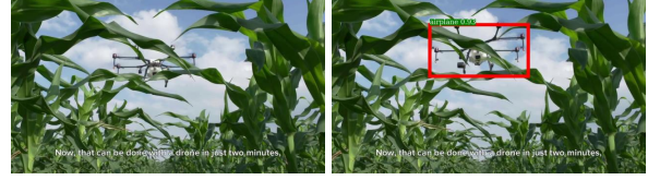
Figure 8: The UAV is occluded in both images but the right one can be detected.
