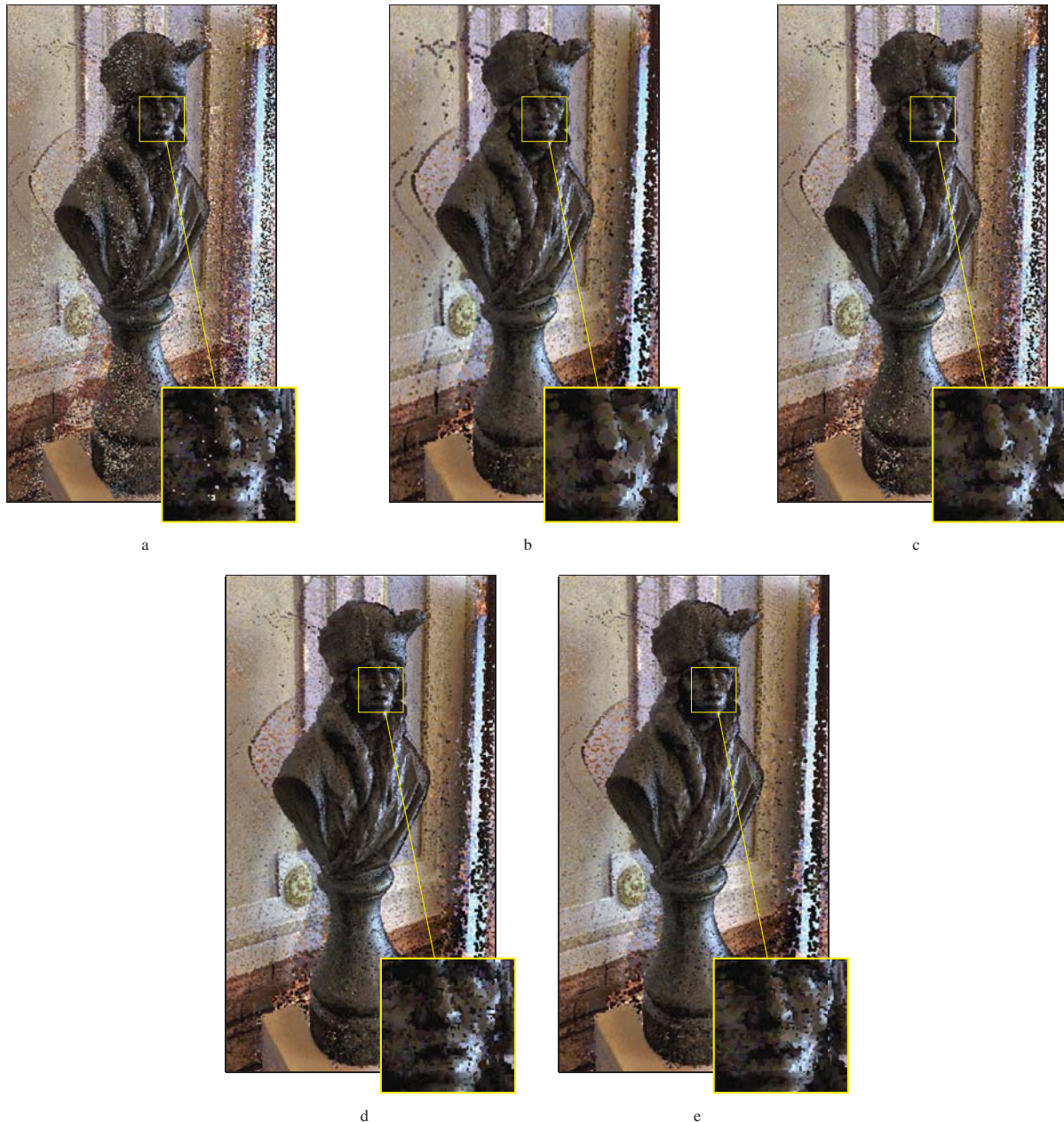
Figure 8: Incorrectly sized points may lead to a holey appearance (a – point size of 1px) or visual clutter (b – point size of 5px). An adaptive point size strikes a balance between both artifact types, but does not eliminate them completely (c). This can be minimized by applying paraboloid rendering (d – diameter of 5px) or filling (e – 5x5 filter kernel and point size of 1px).
