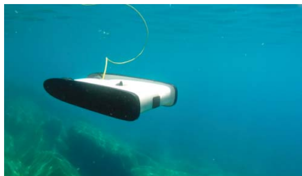
Figure 5: A small underwater OpenROV robot connected through a thin cable for video and control transmissions [16].
