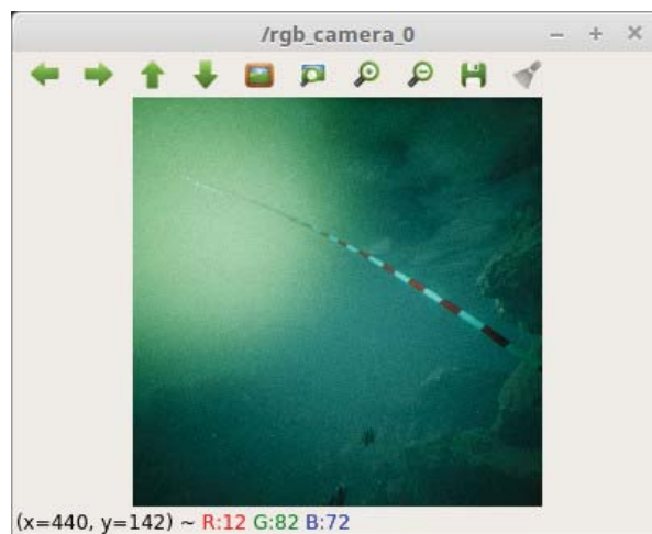
Figure 12: An underwater robot's camera view of its own tether cable
