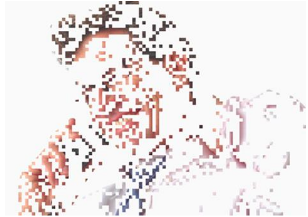
Figure 5. Result of segmentation for \delta = 2 (micro-blocks 4 \times 4 ; Th = 1.5 )
