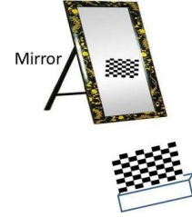
Figure 3: The Kinect camera can see the checkerboard through the mirror
