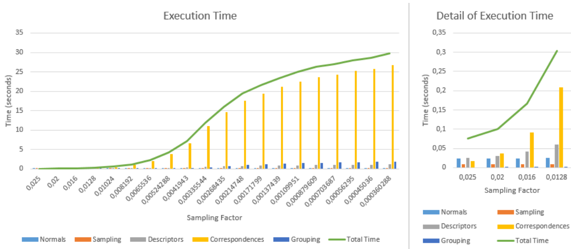
Figure 5: Time of five main task involved in the process of detection
