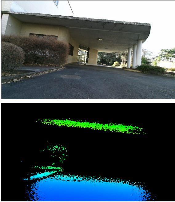
Figure 1: Measurement data from a RGB-D sensor in outdoor scenes. The top shows acquired color image. The bottom shows color mapped depth image. The black colored area represents out of range. The area which is near to the viewpoint is acquired.
