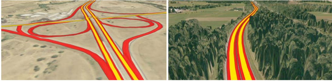
Figure 2: Cartographic rendering of road maps using vivid colors and dark edges to achieve a high visual contrast to the underlying terrain.
