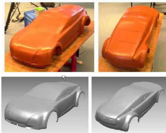
**Figure 8** A 1:5 automotive model (top) was fully automatically registered and merged into a surface model (bottom).
