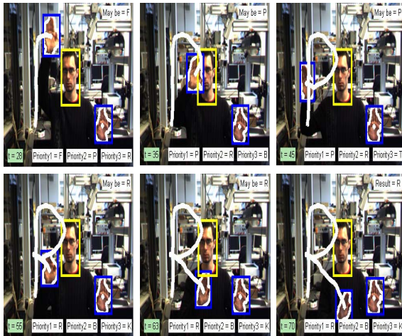
Figure 12. System output for alphabet R, where at t=28 the high priority is alphabet F, at t=45 the high priority is alphabet P and at t=70 the result is R.
