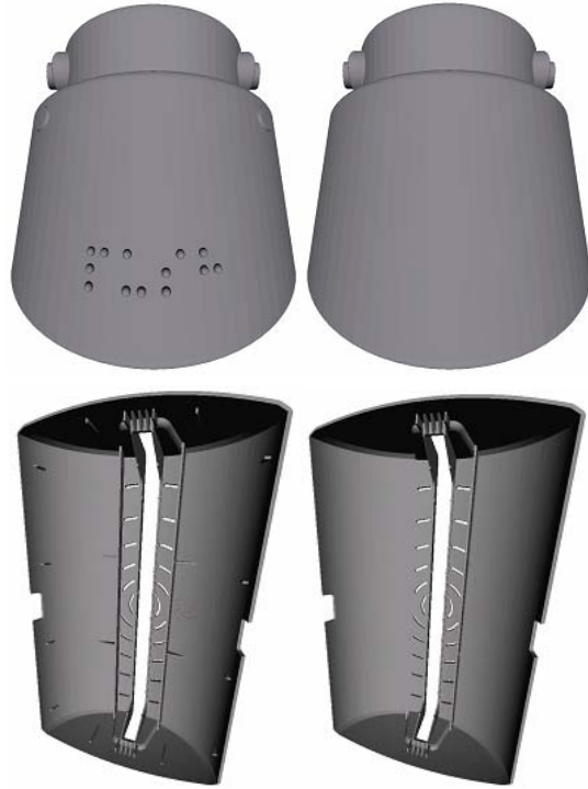
Figure 5: Test models (left) and the result of the feature deletion procedure (right).
