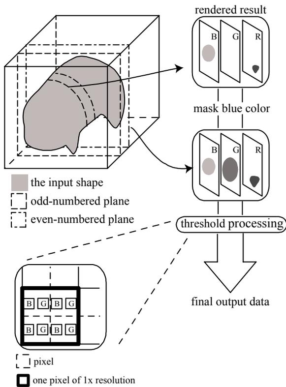
Figure 8. Improving the accuracy of the voxel data
