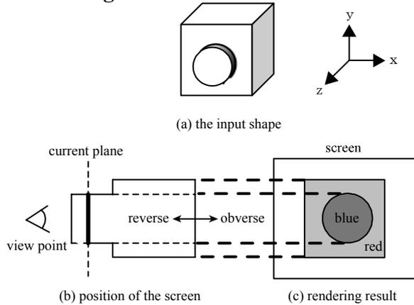
Figure 6. Relation between screen position and drawing result
