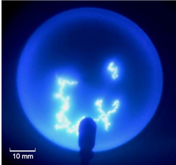
Figure 1b. Photograph of arc spots moving over cylindrical Ti cathode. Exposure time 8 ms.
