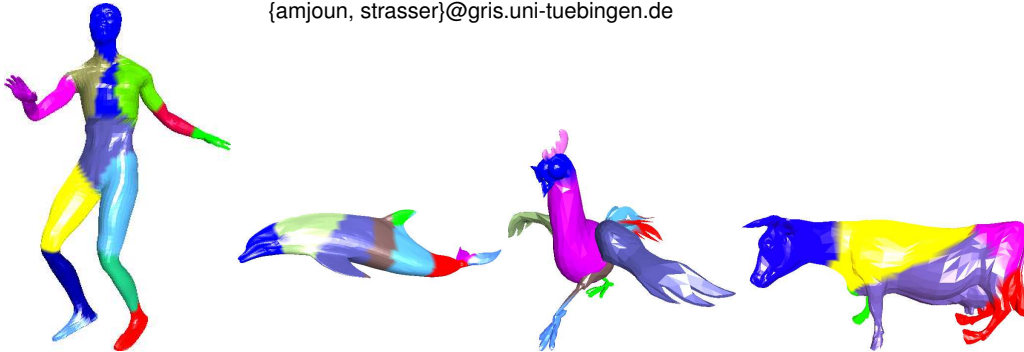
Figure 1 : Sample frames of the animations used for the analysis. From left to right: dance with 14, dolphin with 9, chicken with 10 and cow with 6 clusters. Each cluster is colored differently and encoded separately.
