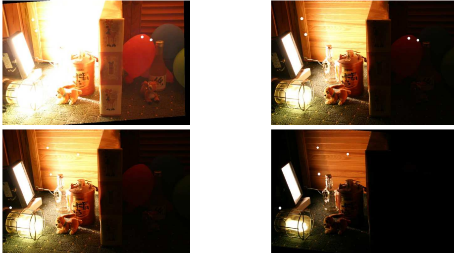
Figure 5: Example photographs taken with a very short and very long exposures. Valid key-points are marked as white dots. There are no key-points in too dark and too light areas.
