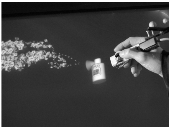
Figure 5: Spraying in the scene with a spray can shaped tool. The icon also reflects the aperture angle of the tool.
