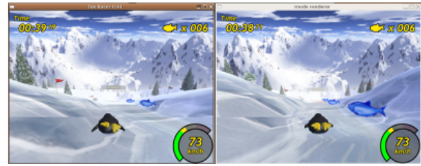
Figure 12: As before, the left indicates the local render, while the right has been transmitted through 4 hops before rendering. Using the rendered timer, the difference can be observed to be about 480ms; on average we found it to be approximately 940ms.
