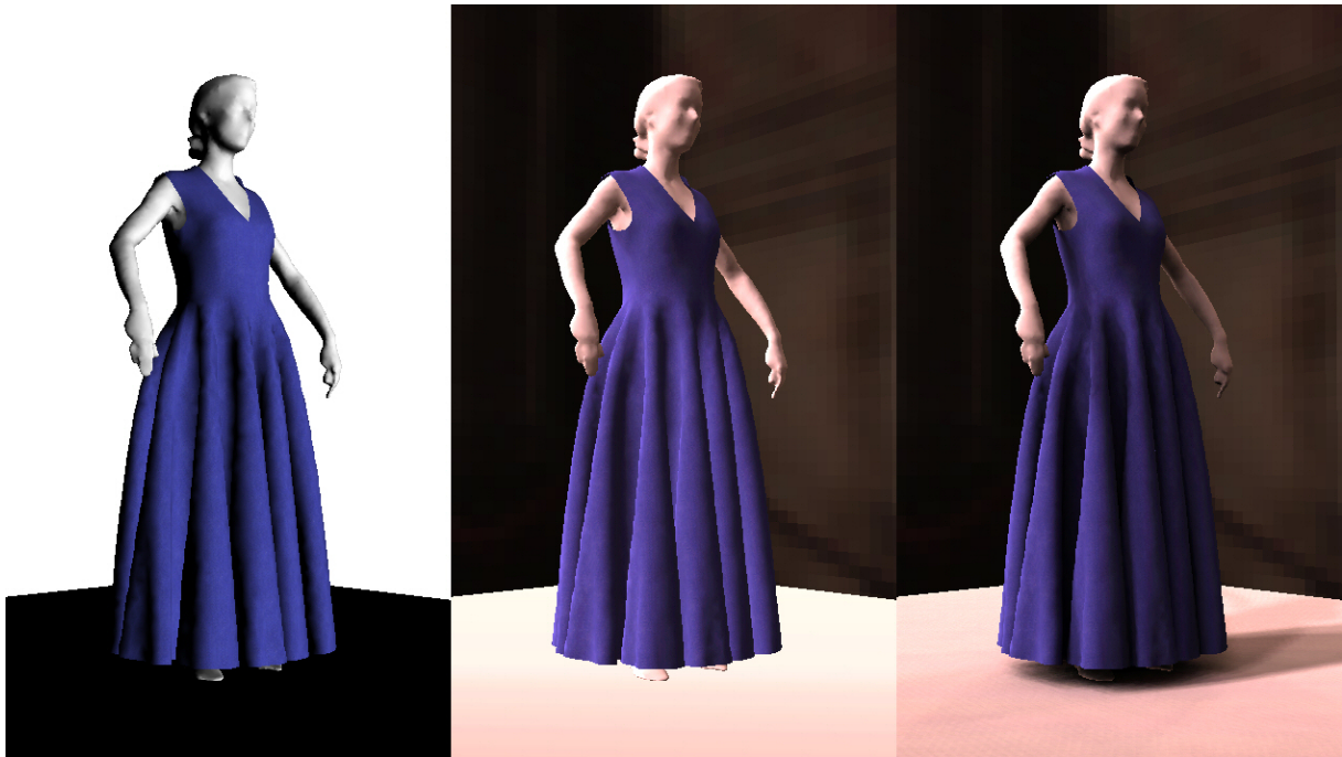
Figure 6: The left image was rendered with standard OpenGL. The center image was illuminated by an irradiance map. The right image was rendered with our algorithm taking self-shadowing into account. The resolution was 421x711 pixel and 128 smoothed shadows were used. We achieved four frames per second. The model consists of 107K triangles.
