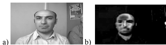
Figure 10. Rescaled source image in RGB color space (a), in I2 color space with normalize step (b)
