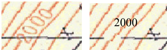
Figure 15. Problems occurred in case of elevation number
