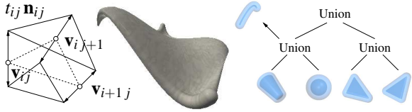
Figure 6: A surface patch with varying thickness primitives, and its corresponding BlobTree representation.
