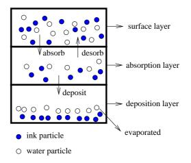
Figure 5. The layer structure of a cell.
