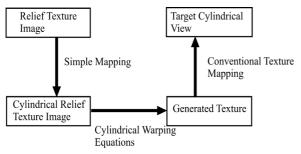
Figure 1. The three-stage mapping process of cylindrical relief texture mapping.
