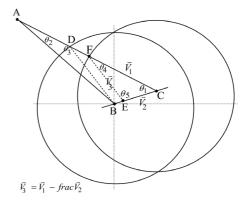
Figure 11. Geometry used for calculating *frac*
