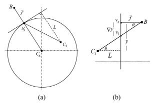
**Figure 6.** The vertical warp calculates point  $b'_s$  vertical shift, that is from  $v_s$  to  $v_i$ , using simple geometry. The amount of shift is dependent on the orthogonal distance from the target viewpoint  $C_t$  to the plane tangent to cylinder at  $b'_s$  (6a) and the associated depth at  $b'_s$ . The geometry used to compute the vertical shift is shown in (6b).
