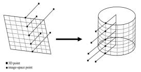
**Figure 2.** Simple mapping from planar to cylindrical relief texture. While the center-of-projection of a planar relief texture is at infinity, a cylindrical relief texture has its center-of-projection at the cylinder axis.
