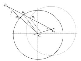
**Figure 5.** The horizontal warp calculates point  $b_s$  shift in the u-direction. A 2D warp, form the reference cylinder with center  $C_s$  to a target cylinder with center  $C_t$ , is carried out to get point  $u_t$ , which is used afterwards to compute  $u_i$ .
