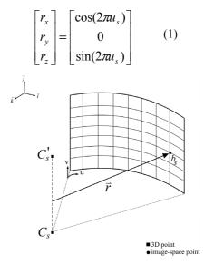
Figure 3. Mapping of cylindrical image-space point  $b_s$  to 3D-space ray r. All points along one image column result in the same 3D ray.
