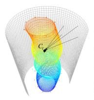
**Figure 9.** Cylindrical relief texture mapping can be used to enhance the realism of endoscopic simulations. A cylinder enclosing the surface is first computed then used in the cylindrical relief texture mapping process.
