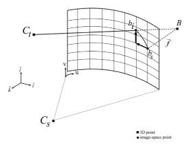
**Figure 4.** The cylindrical warping equations compute the shift of the cylindrical coordinates of point  $b_s$  to new point  $b_i$  induced by the position of target viewpoint  $C_t$  and the depth associated with  $b_s$ .
