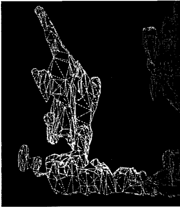
Figure 4: A part of the first smoothed and then decimated pore structure. At this value the reduction of the number of vertices is 77.3 % and the number of triangles is reduced by 77.6 %. After 10 iterations it consists of 130 thousand vertices and 255 thousand triangles.
