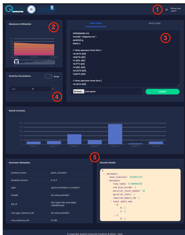
Figure 5: Q-AIM Web User Interface. Users can provide code and runtime parameters in different formats, monitor resource utilization, and visualize results and metadata.
